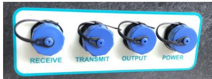
Fig 2.2 the Portable unit Output Interfaces
