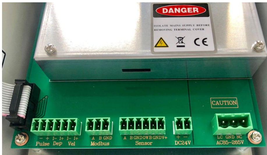
Figure 4.3. Wall-mounted Calculator Wiring Diagram
